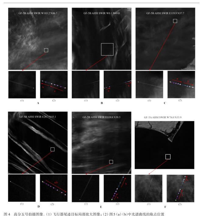
图 4 高分五亏扣摄图家。(1) 飞行器电迹目标同部放入图家; (2) 图 5 (a) (b) 中尤谓曲线的取点位直 Fig. 4 Gaofen-5 satellite imagery. (1) Zoomed-in image of the aircraft-contrail target; (2) Sampling point locations of the spectral curve in Fig. 5 (a) and (b)
