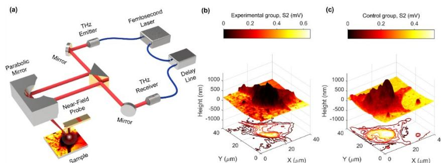
Fig. 1 Schematic of THz near-field nano-imaging experiments on MEFs. : (a) Experimental set-up; (b,c) Topological morphology (AFM) and second-order THz near-field amplitude (S2) of MEFs. (b) Experimental group; (c) Control group
