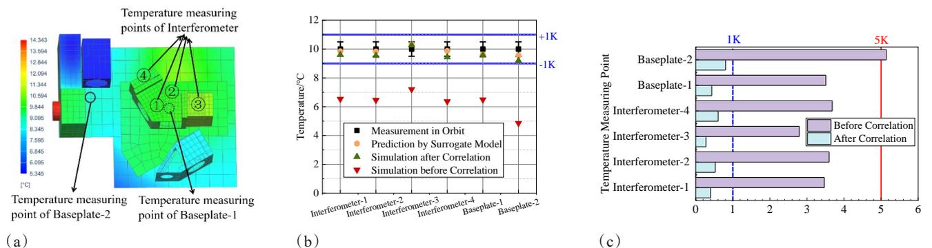
Figure 5 Correlation result of cold case for FY-3E/HIRAS-II: (a) Temperature cloud map (b) Correlation results of temperature comparison (c) Absolute error
