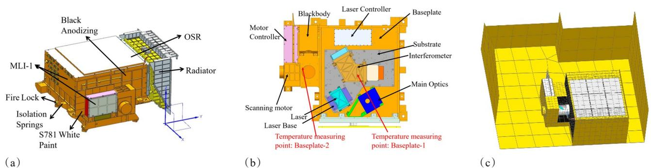
Figure 1 Model of FY-3E/HIRAS-II: (a) Physical model and thermal control measures (b) Distribution of internal components and measuring point of baseplate (c) Mesh of the thermal model for FY-3E/HIRAS-II
