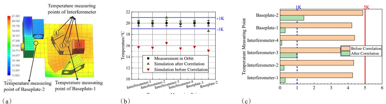
Figure 6 Correlation result of hot case for FY-3E/HIRAS-II: (a) Temperature cloud map (b) Correlation results of temperature comparison (c) Absolute error
