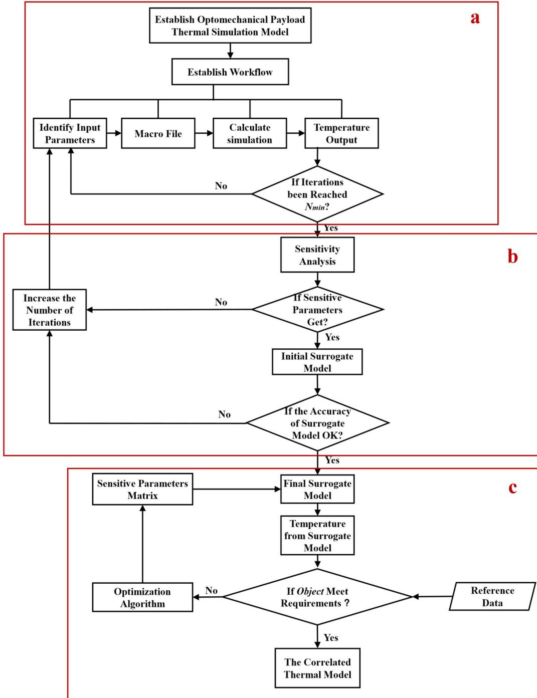
Figure 2 Flowchart of ICP-TM; a. Establish a Workflow.
