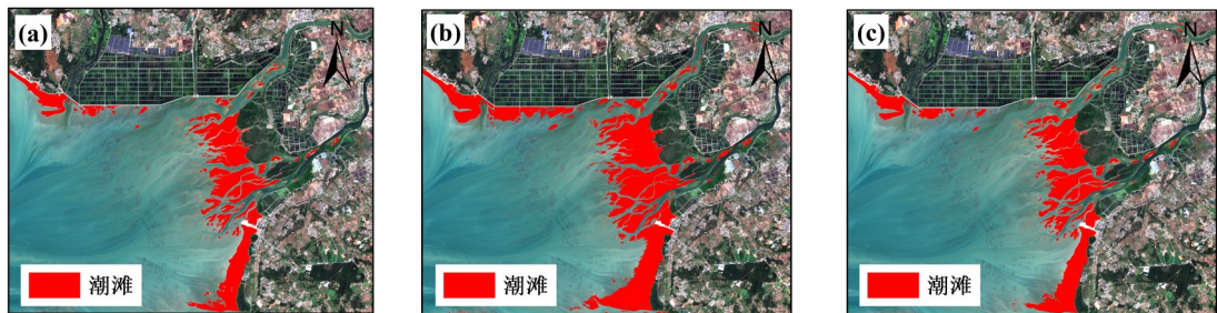
图7 三种分类方法潮滩结果图。(a)最小距离法;(b)极大似然法;(c)支持向量机 Fig. 7 Tidal flat results of three classification methods. (a) Minimum Distance Classification; (b) Maximum Likelihood Classification; (c) Support Vector Machine
