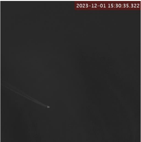
图 21 晴朗天气下线性倍增模式对飞机成像图 1 Fig. 21 Imaging of aircraft by linear multiplication mode in clear weather 1
