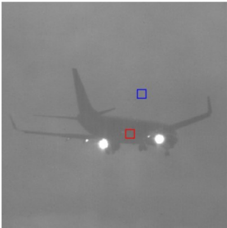
图 20 阴雨条件下雪崩模式飞机成像图 Fig. 20 Avalanche mode aircraft imaging under cloudy and rainy conditions
