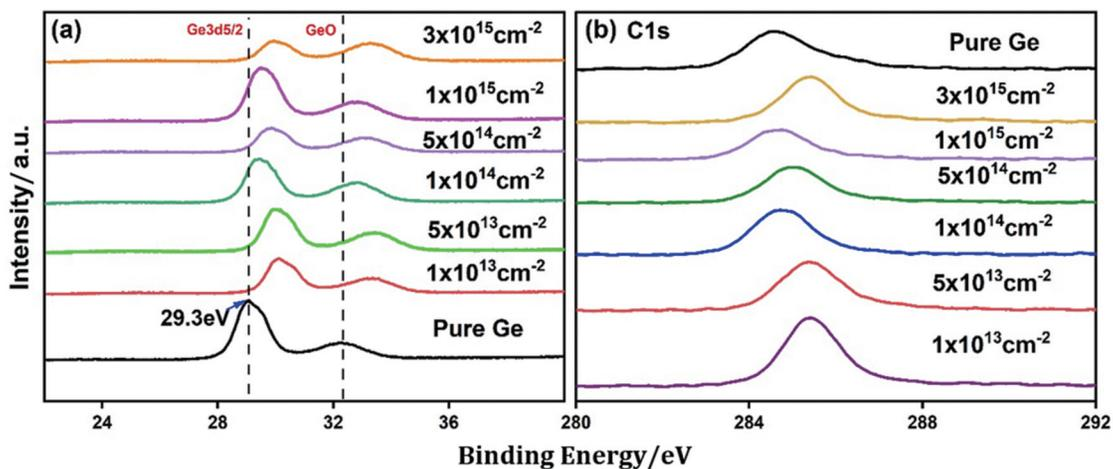
Fig. 4 XPS spectra illustrating boron implantation into germanium across distinct doses: (a)  $\text{Ge}^{3d}$  scan; (b)  $\text{C}^{1s}$  scan
