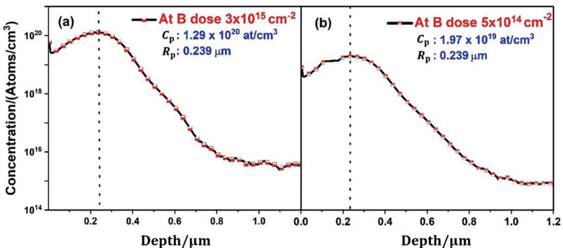
Fig. 6 SIMS analysis of B implanted Ge for two high doses: (a)  $3 \times 10^{15} \text{ cm}^{-2}$ ; (b)  $5 \times 10^{14} \text{ cm}^{-2}$
