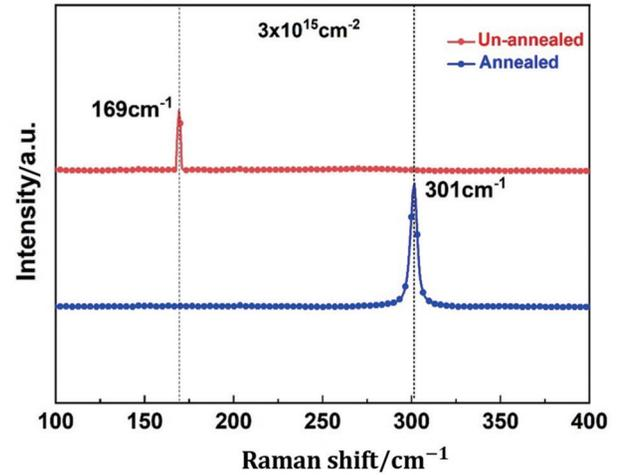
Fig. 3 Raman spectra of the germanium samples implanted at  $3 \times 10^{15} \text{ cm}^{-2}$  before and after annealing
