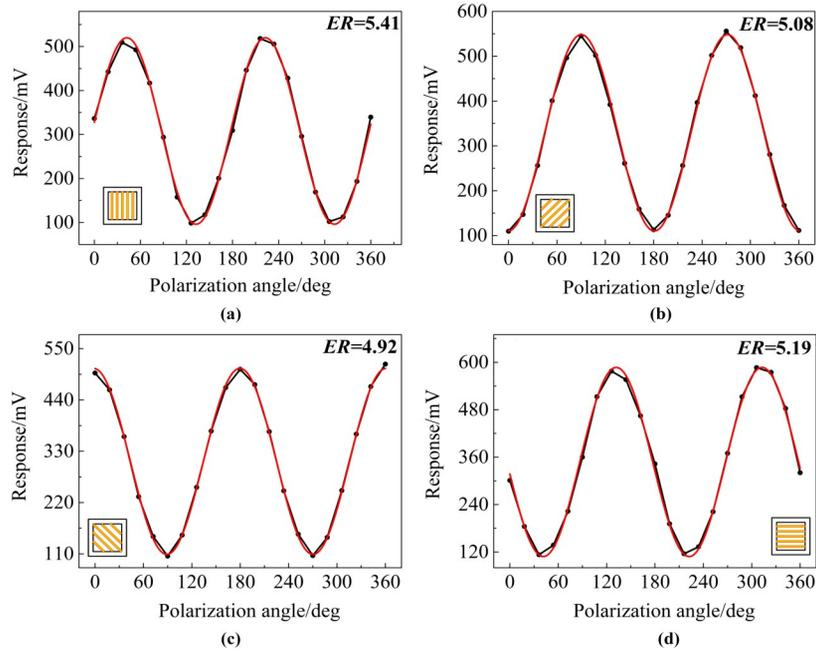
Fig. 12 Polarization response curves of pixels with (a-d) 0°, 45°, 90°, and 135°orientations for the A-type polarimetric FPA
