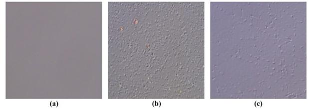
Fig. 5 Surface morphologies of Au layers fabricated by: (a) e-beam evaporation; (b) magnetic sputtering; (c) ion beam sputtering
