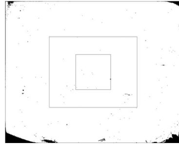
Fig. 11 Blind pixel distribution diagram of the polarimetric FPA after the preliminary process optimization
