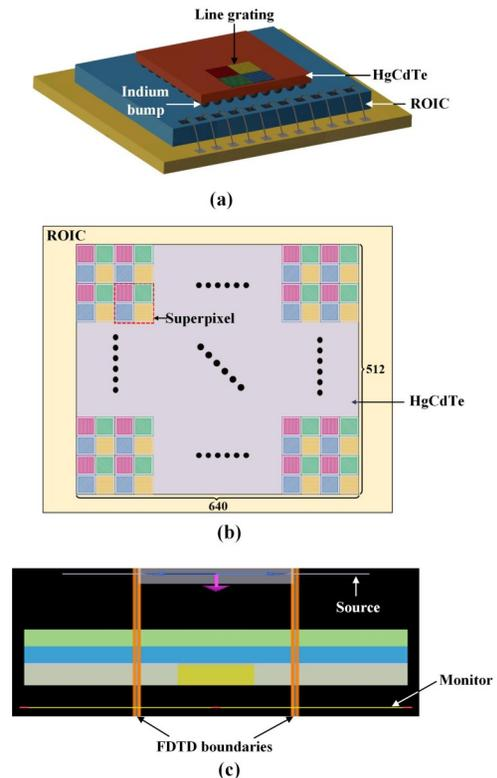
Fig. 1 Monolithic polarimetric FPA: (a) the schematic of a monolithic polarimetric FPA; (b) the arrangement of superpixels; (c) the established model to optimize structural parameters
