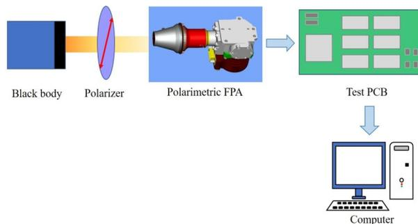
Fig. 9 Test setup of the polarimetric FPA
