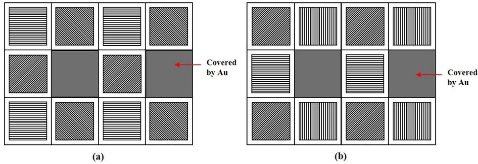
Fig. 15 Specialized MPA layout to determine crosstalk rates from adjacent pixels of (a) 0°- and (b) 45°- oriented pixels
