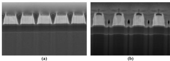
Fig. 7 Cross-sectional profiles of etched line gratings before (a) and after (b) process condition modifications
