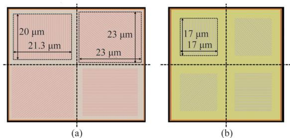
Fig. 3 MPA layout: (a) the previously reported MPA layout; (b) the modified one with expanded opaque regions
