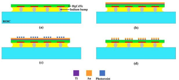
Fig. 4 MW 640 × 512 (25 μm) HgCdTe FPA: (a) monolithic integration process; (b) Ti/Au depositions; (c) laser direct writing; (d) iron-beam milling
