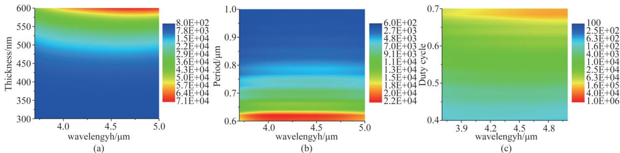
Fig. 2 *ER* variation tendencies with respect to different structural parameters: (a) thickness; (b) period; (c) duty cycle
