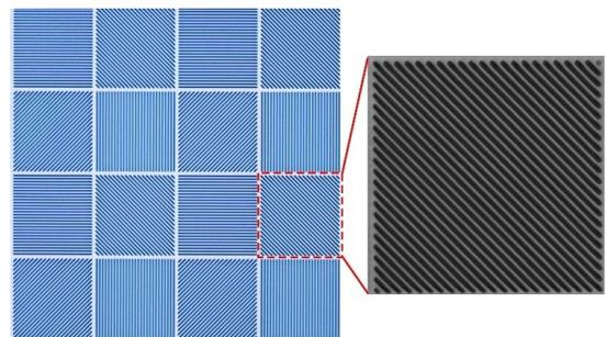
Fig. 6 Patterned line gratings with optimal process parameters of laser direct writing
