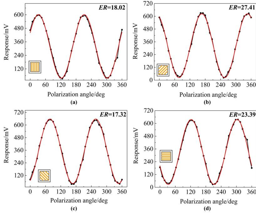
Fig. 14 Polarization response curves of pixels with (a-d)  $0^\circ$ ,  $45^\circ$ ,  $90^\circ$ , and  $135^\circ$  orientations for the formally encapsulated B-type polarimetric FPA
