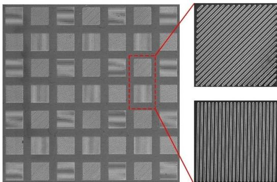
Fig. 8 SEM photographs of the monolithically fabricated MPA
