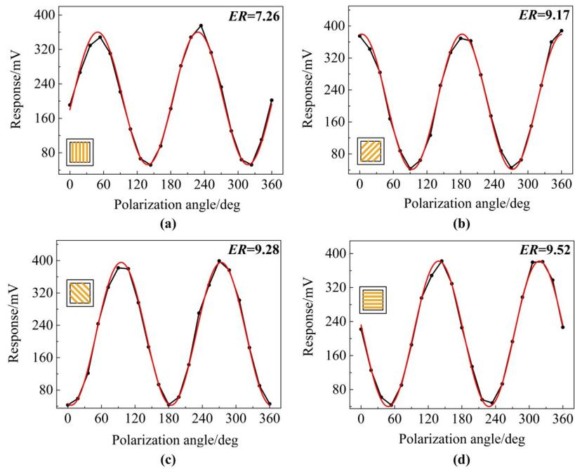
Fig. 13 Polarization response curves of pixels with (a-d) 0°, 45°, 90°, and 135°orientations for the B-type polarimetric FPA
