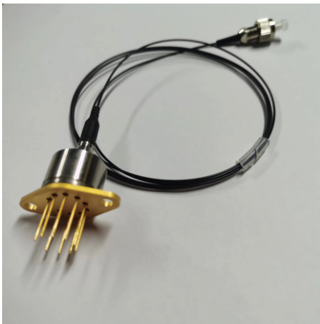
Fig. 4 Physical appearance of an InGaAsP/InP SPAD 图 4 InGaAsP/InP SPAD 的物理外观
