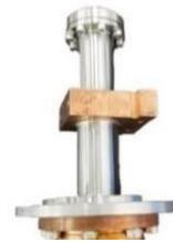
Fig. 3 Photo of 15 K second-stage pulse tube cryocooler
