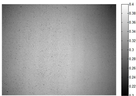
图5 77 K下 x_{Cd}=0.205 的甚长波器件响应率灰度图 Fig. 5 Responsivity pixel map for a VLWIR FPA with x_{Cd}=0.205 at 77 K
