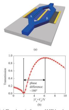
Fig. 4 (a) The schematic diagram of MZI based on optimized GEW ( $W_{\text{GEW}}$ =800 nm,  $H_{\text{GEW}}$ =100 nm), (b) Transmission of MZI based on the optimized GEW as a function of the applied voltage  $|V_x + V_0|$
