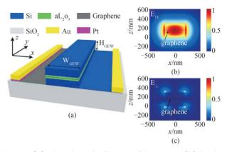
Fig. 1 (a) The schematic diagram of the GEW, (b) in-plane electric field distribution for TE mode, and (c)out-of-plane electric field distribution for TE mode
