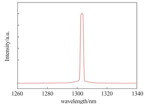
Fig. 5 Lasing spectrum at RT (The central wavelength is 1.3  $\mu\text{m}$ )
