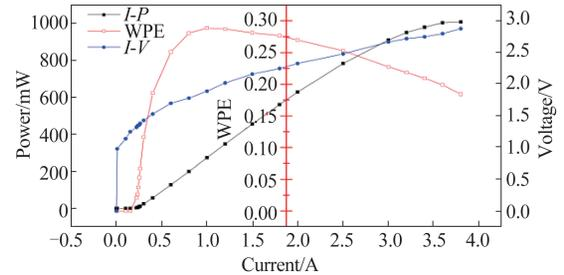
Fig. 4  $P$ - $I$ - $V$  and WPE characteristics of the laser at CW mode
