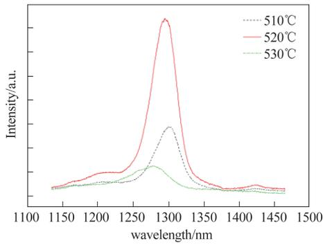
Fig. 2 PL spectrum of the three QDs samples with growth temperature of 510°C, 520°C and 530°C
