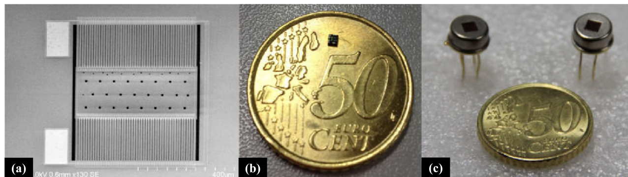
图2 MEMS热电堆红外探测器:(a)芯片电镜图;(b)裸芯片;(c)封装后器件 Fig. 2 MEMS thermopile IR detector:(a) SEM image of chip; (b)Bare chip; (c)Packaged detector
