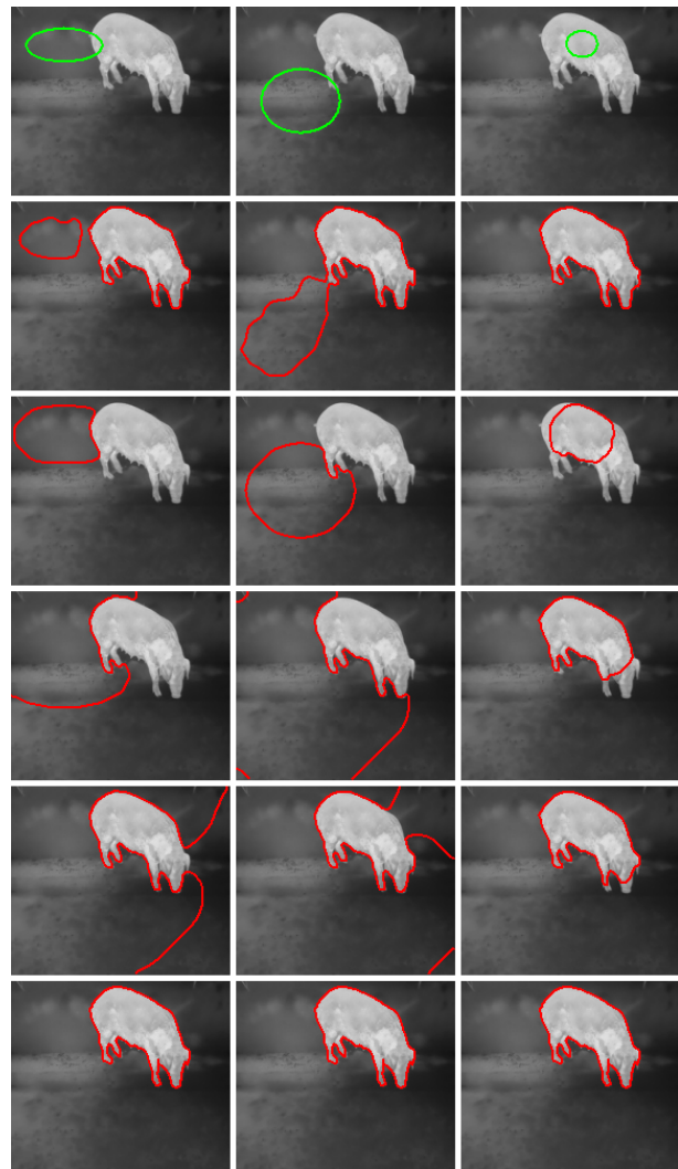
Fig. 8 Segmentation comparisons of our model with LBF model on an infrared pig image under three different initializations. The first row: Input images along with initial contours; the second row: Final segmentation results of LBF model; the third to fifth rows: Three intermediate results of our model; the sixth row: Final segmentation results of our model
