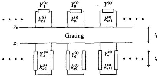
Fig. 3 Equivalent multimode network representation of the grating antenna.
