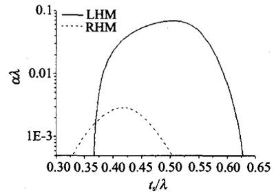
Fig. 5 Variation of leakage constant with substrate thickness.  $t_g = 0.05\lambda$ ,  $d_1 = d_2 = 0.5d$ ,  $d = 0.6\lambda$  ( $\lambda = 1.0$ )
