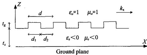
Fig. 1 The structure of LHM periodic grating leaky wave antenna and related parameters.
