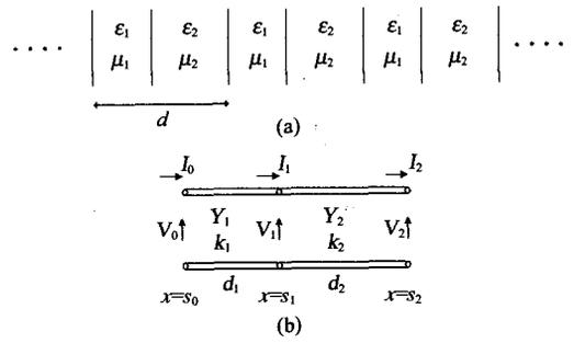
Fig. 2 (a) Infinite periodic dielectric layers. (b) Equivalent transmission line model of unit cell.
