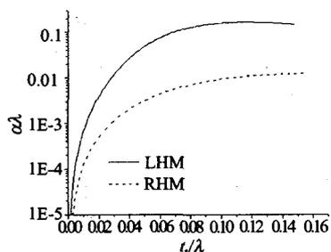
Fig. 6 Variation of the leakage constant with grating thickness.  $tg = 0.4\lambda$ ,  $d_1 = d_2 = 0.5d$ ,  $d = 0.6\lambda$  ( $\lambda = 1.0$ )
