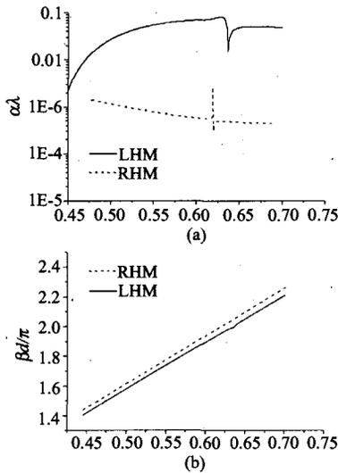
Fig. 4 (a) Variation of leakage constant with grating period. (b) variation of phase constant with grating period.  $d_1 = d_2 = 0.5d$ ,  $t_s = 0.45\lambda$ ,  $t_g = 0.05\lambda$  ( $\lambda = 1.0$ ).
