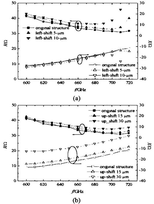
Fig. 5 Embedding impedance simulated for different feed point displacements
