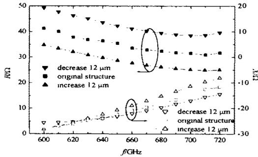
Fig.7 Embedding impedance simulated for different backshort lengths
