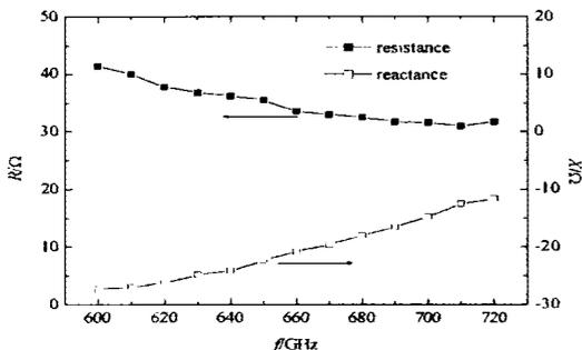
Fig. 4 Embedding impedance as a function of frequency
