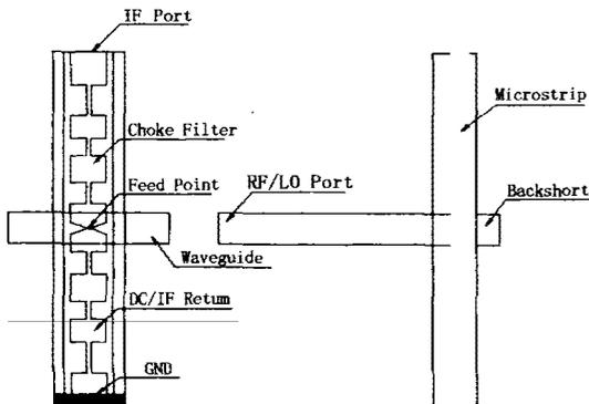
Fig. 1 Geometry of a 600-720GHz SIS mixer mount
