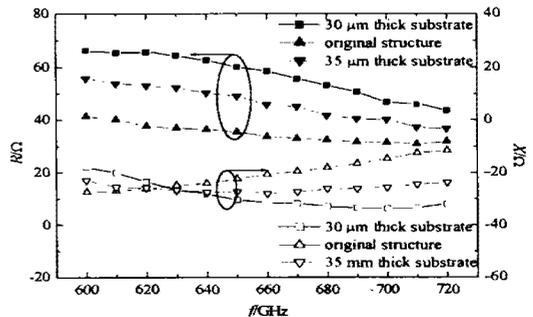
Fig. 6 Embedding impedance simulated for different junction chip thicknesses
