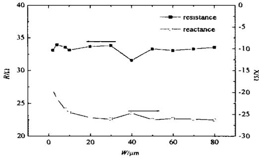
Fig. 3 Embedding impedance at 600GHz vs feed point width
