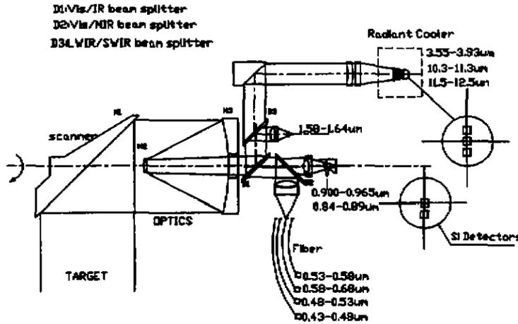
Fig. 3 The optical system of the scanning radiometer
