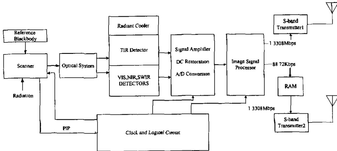
Fig. 2 Block diagram of the 10-band scanning radiometer
