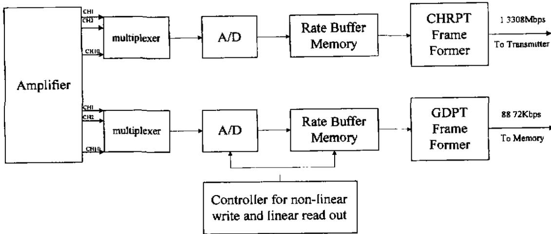
Fig. 5 Image signal processor configuration
