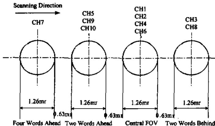
Fig. 4 The arrangement of 10 bands' IFOV
