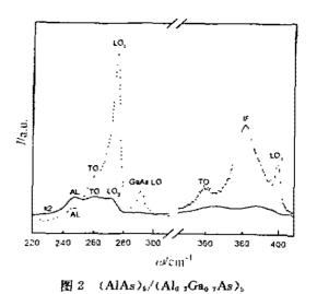
超晶格的室温喇曼散射光谱 Fig. 2 The room-temperature Raman spectra of (AlAs)<sub>5</sub>/(Ala<sub>3</sub>Ga<sub>2</sub>As)<sub>5</sub> superlattices
