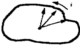
图 1 径向矢量表示的边界 Fig. 1 Shape representation by radius vectors
