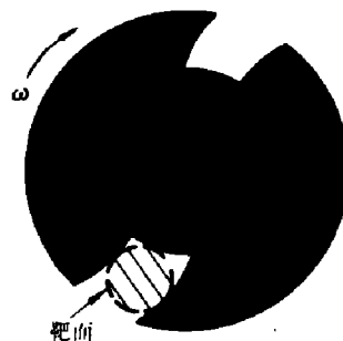
图 6 非对称斩波盘形状 Fig. 6 The shape of the chopper used in the asymmetrical mode
