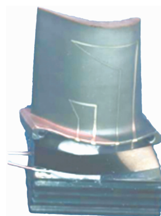
图2 美国第4宇航局在涡轮叶片上制备的薄膜热电偶 Fig.2 The thin-film thermocouple produced on turbine blades by NASA [4]
