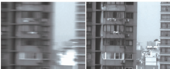
图7 翼展摆扫单帧成像的像移补偿前后效果对比图 Fig.7 Before-and-after compensation of one frame image in wingspan pendulum sweeping process
