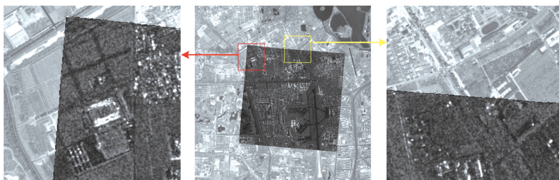
图7 5°旋转图像间级联变换配准结果及细节展示 Fig.7 Details of cascade transform registration with 5° rotation
