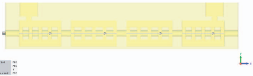
图 8 三维注波相互作用仿真模型 (CST Particle Studio) Fig. 8 Model for the three-dimension interaction simulation in the CST Particle Studio
