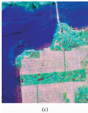
Fig. 2 Decompositions of AIRSAR data on San Francisco with m_s for blue, m_d for red, m_v for green. (a) Original hybrid Freeman/eigenvalue decomposition, (b) Hybrid Freeman/eigenvalue decomposition with extended volume scattering model, (c) Proposed hybrid Freeman/eigenvalue decomposition
