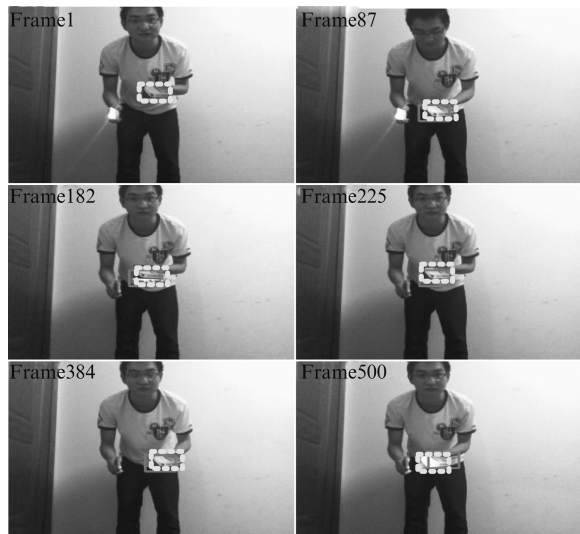
图3 利用 Compressive Tracking 算法对 Tang 视频序列的跟踪效果 Fig. 3 Tracking results of Tang video sequences by compressive tracking algorithm
