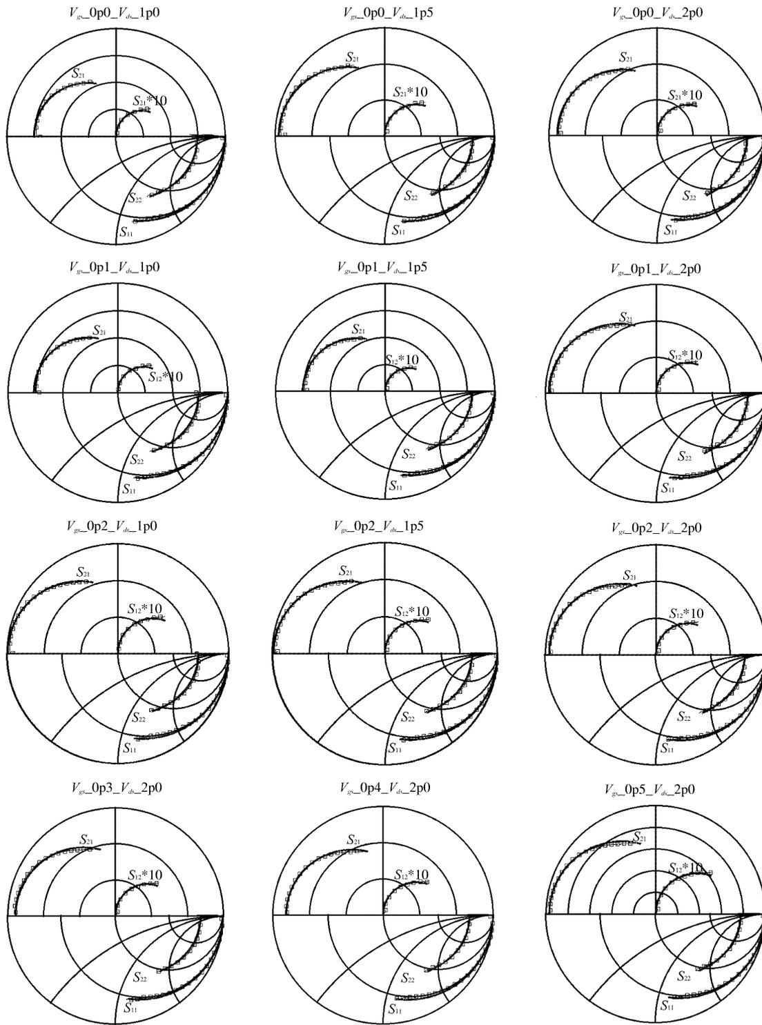
Fig. 5 Modeled and measured s-parameters for HEMT under different bias
