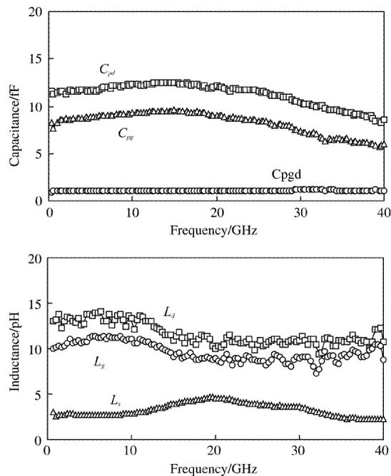
Fig. 4 Pad Capacitances and parasitic inductances extracted from test structure
