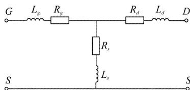
Fig. 3 Parasitic inductances equivalent circuit of short test structure
