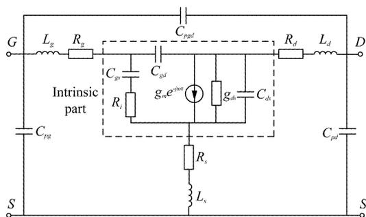
Fig. 1 Small-Signal Equivalent Circuit of HEMT
