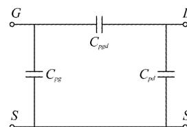
Fig. 2 Pad capacitances equivalent circuit of open test structure
