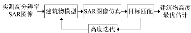
图 9 基于仿真图像匹配的建筑物高度提取流程图 Fig. 9 Flowchart of building height estimation based on iterative simulation and matching
