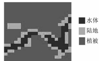
图10 地表分类图 Fig. 10 classification image(water, land and vegetation)
