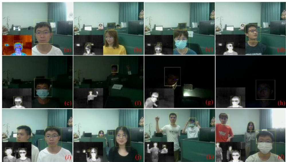
Fig. 5 IR face detection samples of YOLO-Fastest-IR and eye localization in the RGB images results: (a~d) YOLO-Fastest-IR and YOLO-Fastest-Eye are robust against variations in face angle, inter-viewer occlusion, and environmental occlusion; (e~h) extreme lighting conditions; (i~l) multi-target and distant viewer detection 图5 YOLO-Fastest-IR 热红外人脸检测结果及在RGB图像中人眼定位效果:(a~d) YOLO-Fastest-IR 与 YOLO-Fastest-Eye 对脸部角度变化、观察者间遮挡及环境遮挡具有鲁棒性;(e~h) 极端光照条件;(i~l) 多目标及远距离观察者检测
