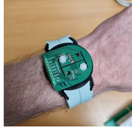
Fig. 6 The front side of the watch-like prototype for measuring wrist temperature
