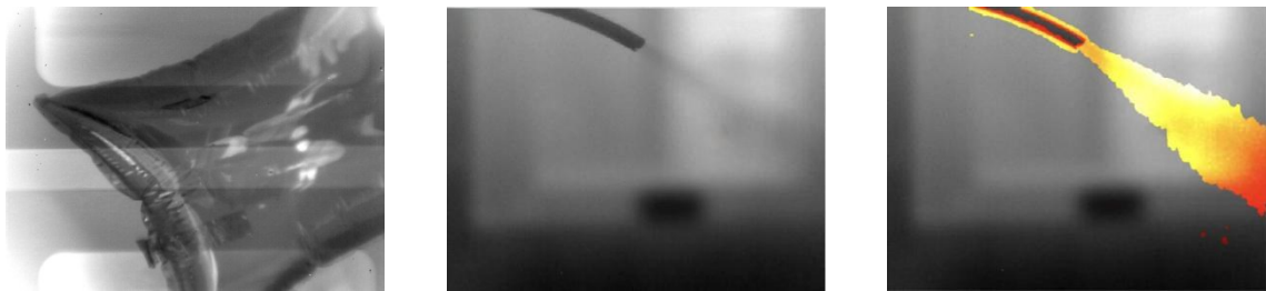
图10 乙烯气体最低检测浓度成像实验 Fig. 10 Imaging experiment of the lowest detection concentration of ethylene gas
