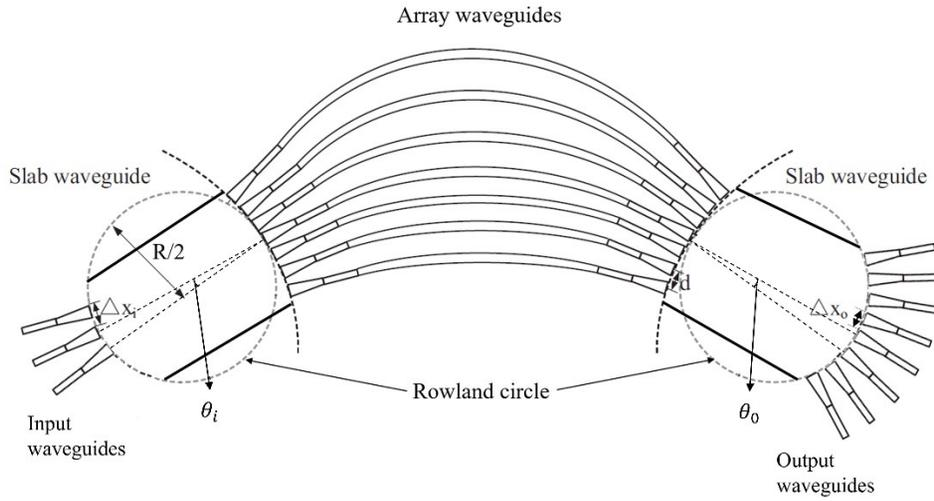
Fig. 1 The schematic structure of the AWG.
