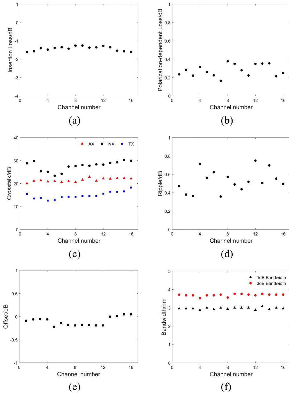
Fig. 10 (a) insertion loss for each channel (b) polarization-dependent loss (c) crosstalk (d) ripple (e) offset (f) bandwidth.
