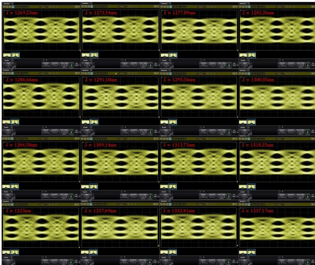
Fig.11 (a) Experimental setup for testing eye diagrams and (b) the measured 53.125 GBaud PAM4 optical eye diagrams for all channels: 图十一 (a)测试眼图的实验装置图(b)所有通道的 53.125 GBaud PAM4 光眼图测量结果
