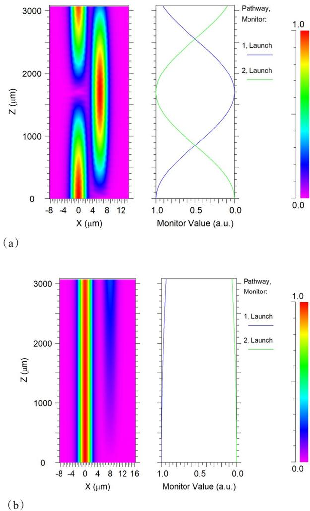
Fig. 3 (a) Simulated mode field propagation at  $6 \mu\text{m}$  spacing (b) Simulated mode field propagation at  $8 \mu\text{m}$  spacing
