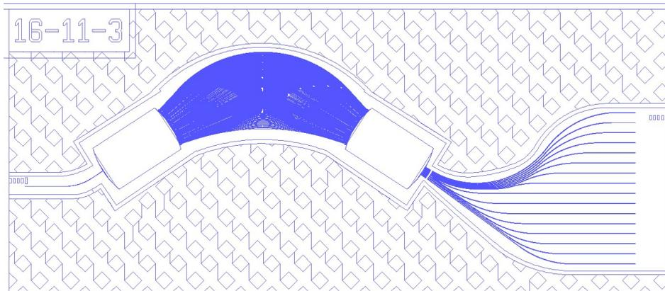
**Fig. 6 The schematic of 16-channel AWG**
