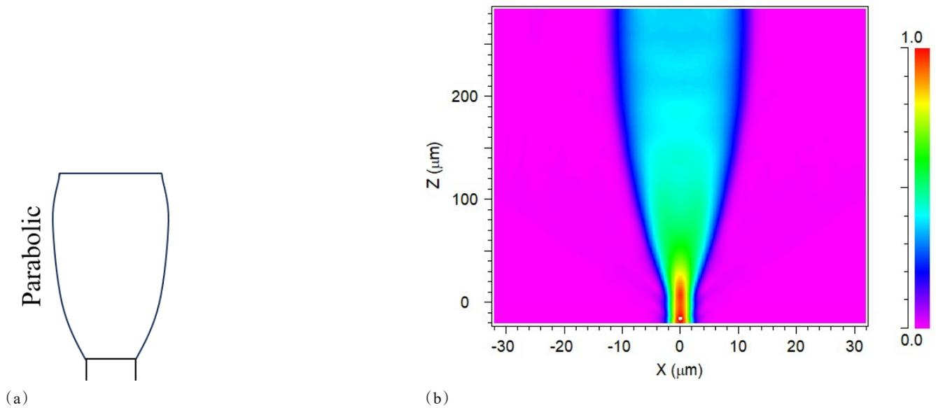
Fig. 4 (a)The top view of a parabolic taper. (b) Parabolic tapered waveguide transmission field
