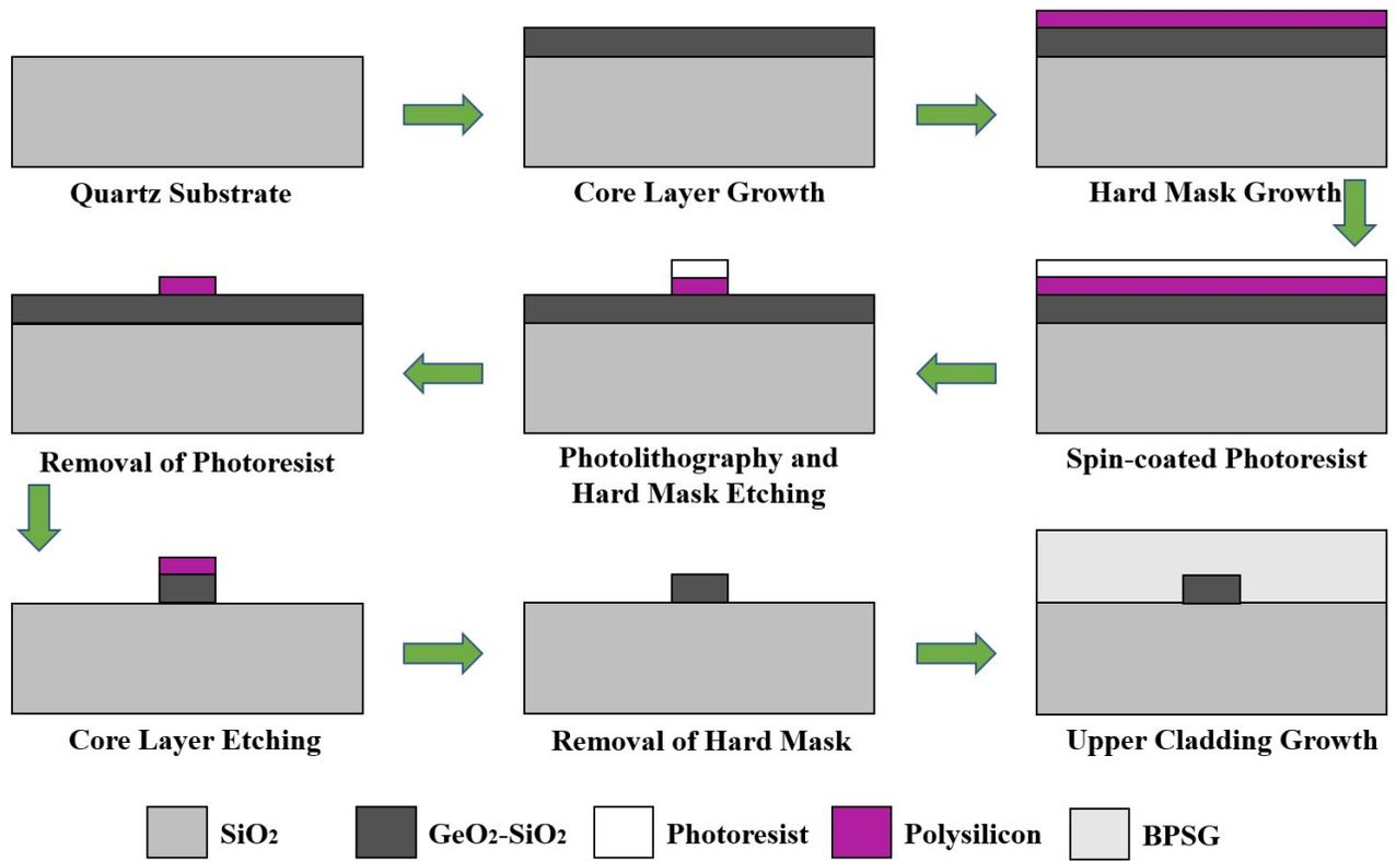
Fig. 7 The schematic diagram of the 16-channel AWG fabrication process
