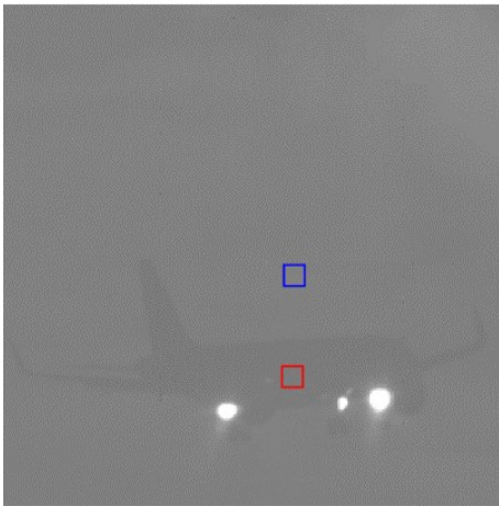
图19 阴雨条件下常规模式飞机成像图 Fig. 19 Conventional mode aircraft imaging under cloudy and rainy conditions
