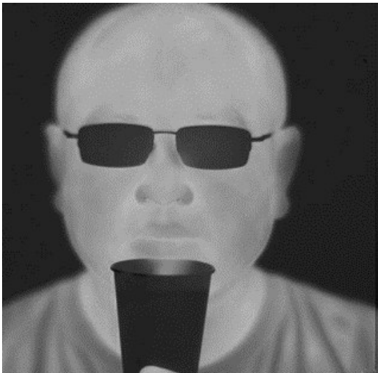
图 7 百万像素长波探测器高清晰成像图 Fig. 7 High definition image of megapixel long-wavelength detectors
