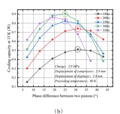
Fig. 4 (a)Effect of frequency on 15 K rCOP, (b)Effect of frequency on 15 K cooling capacity 图 4 (a) 15 K 时频率对 rCOP的影响, (b) 15 K 时频率对制冷量的影响
