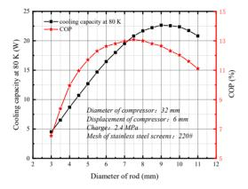
Fig. 6 Influence of the diameter of the push rod on Stirling cryocooler
