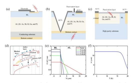
Fig. 12 (a) Structure of topside-illuminated (TSI) vertical BIB detectors, (b) structure of back-illuminated (BSI) vertical BIB detectors, (c) structure of ion-implanted BIB detectors, (d) detector band diagram under positive bias with thermal incidence, (e) electric field intensity as a function of position at different temperatures, (f) the relationship between the depletion region width with temperature.
