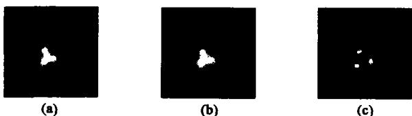
图 6 (a),(b) 序列湍流退化图像, SNR = 20 dB, (c) 复原图像 Fig. 6 (a),(b) A series of turbulence-degraded images in case of SNR = 20 dB, (c) the restored image
