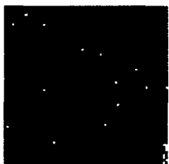
图 5 由 STD 得到的过热像元集合 Fig.5 The over hot pixel set based on the STD characteristic
