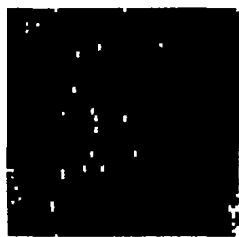
图 4 由 DOM 得到的死像元集合 Fig.4 The dead pixel set based on the DOM characteristic
