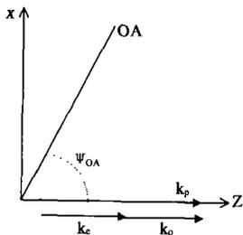
Fig. 1 Collinear perfect phase matching: OA, optic axis of the crystal, lies in the x-z plane
