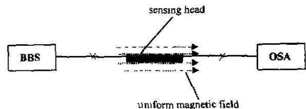
Fig. 2 Schematic diagram of experimental setup for the measurement of current effect
