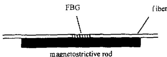
Fig. 1 FBG sensing head
