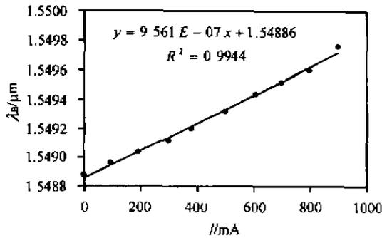
Fig. 3 The relationship between the Bragg wavelength  $\lambda_B$  of FBG and electric current  $I$
