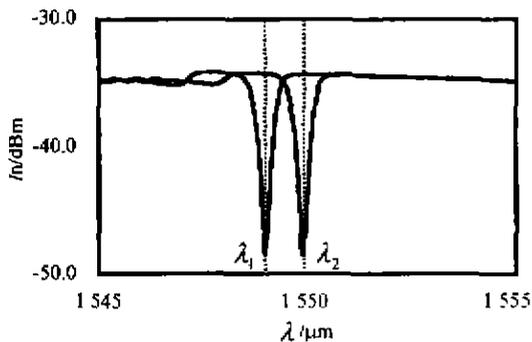
Fig. 4 The transmission spectra of FBG at different electric current
