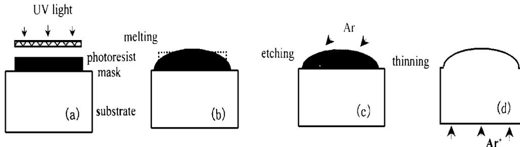
Fig. 2 Fabrication procedures to get the refractive microlens array
