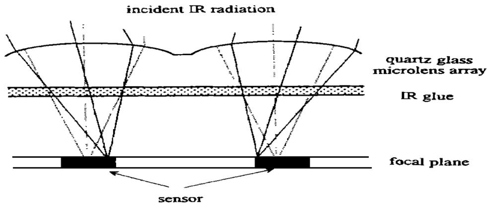
Fig. 5 The schematic cross section of two-pixel architecture of the IR FPAs device with refractive microlens
