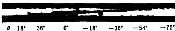
图 2 单面扩硼铝片的应力光弹图 Fig. 2 Stress photoelasticity pattern of boron-diffused aluminium sample in one side
