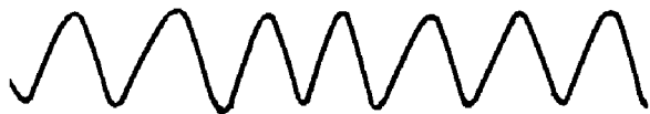
图 6 探测器对 1 GHz 正弦波调制光讯号的响应 Fig. 6 1 GHz sinuous optical signal response for integrated lensed pin PD
