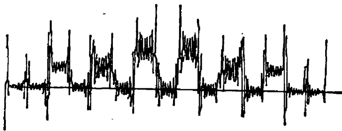
图3 不用窗函数时用解卷积处理重现的目标分布 Fig. 3 Radiation distribution of targets retrieved by deconvolution processing without using window function
