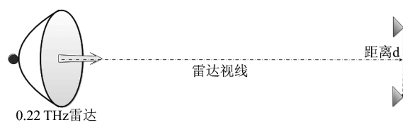
图8 角反射器组 RCS 测试场景示意图 Fig.8 Scene view of RCS measurement model for corner reflectors group
