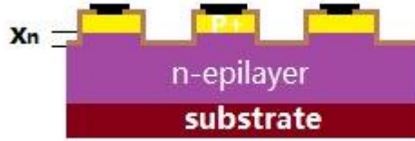
Figure 1. Cross section of an ideal mesa etched variable-area diode array with deep mesa
