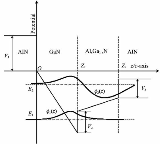
Fig. 1 Schematic diagram of confined potential profile and electronic wave-functions of the ground-state  $\phi_1(z)$ , and the first-excited state  $\phi_2(z)$  in  $z$ -direction of the wurtzite GaN-based step QW
