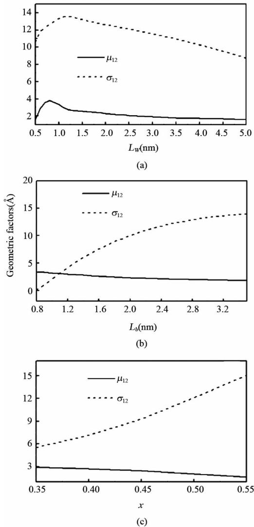
Fig. 2 Geometric factors  $\mu_{12}$  (solid lines) and  $\sigma_{12}$  (dash lines) of the GaN-based step QWs as functions of the well width  $L_w$  [Fig. 2 (a)], the central step barrier width  $L_b$  [Fig. 2 (b)] and the doped concentration  $x$  of the step barrier [Fig. 2(c)]
