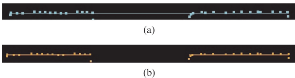
Fig. 5 The discretization of line segments by component analysis (a) Fitting line segment before component analysis, (b) Fitting line segments after component analysis
