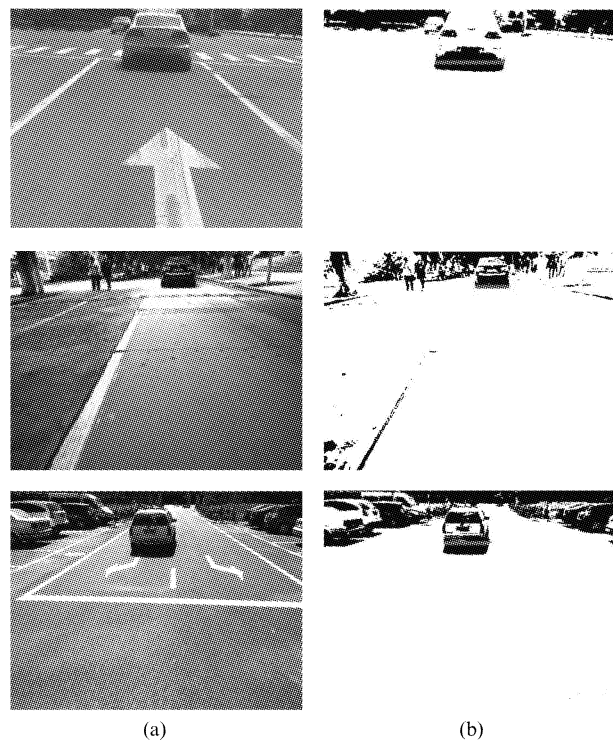
Fig. 8 Results of bottom shadow segmentation based on the improved segmentation algorithm. (a) Original images under different scenarios. (b) Segmentation Results of bottom shadow of vehicle; the green coarse line shows the bottom shadow of vehicle
