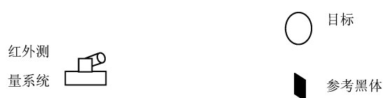
图1 基于实时标校的辐射测量方法原理 Fig.1 Method of radiation measurement based on real-time radiation correction
