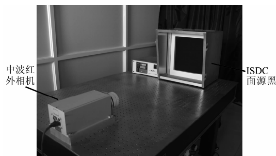
图2 中波红外相机定标示意图 Fig.2 Schematic diagram of radiation calibration of the MW IR camera
